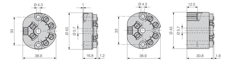
Fig. 4. SINEAX VK 616-71/73, input/output not electrically isolated.
